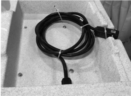
**Ocho Rios SE:** When standing at the topside control panel, the power cord is mounted to the base underneath the topside control panel.
