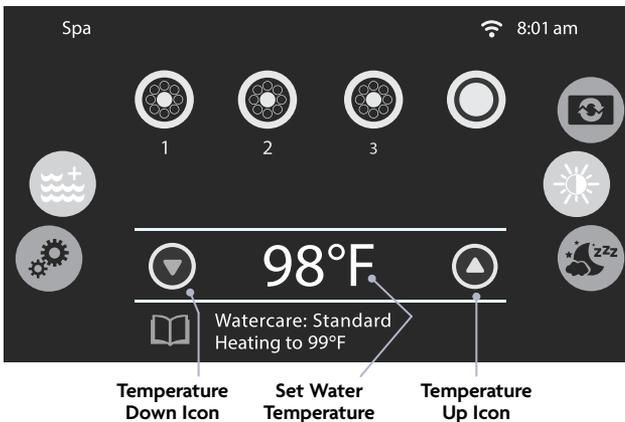
\*Standard systems do not have physical capabilities of cooling the water. Water cooling and achieving lower set temperature will be dependent on ambient conditions and equipment runtime such as filtration durations.
